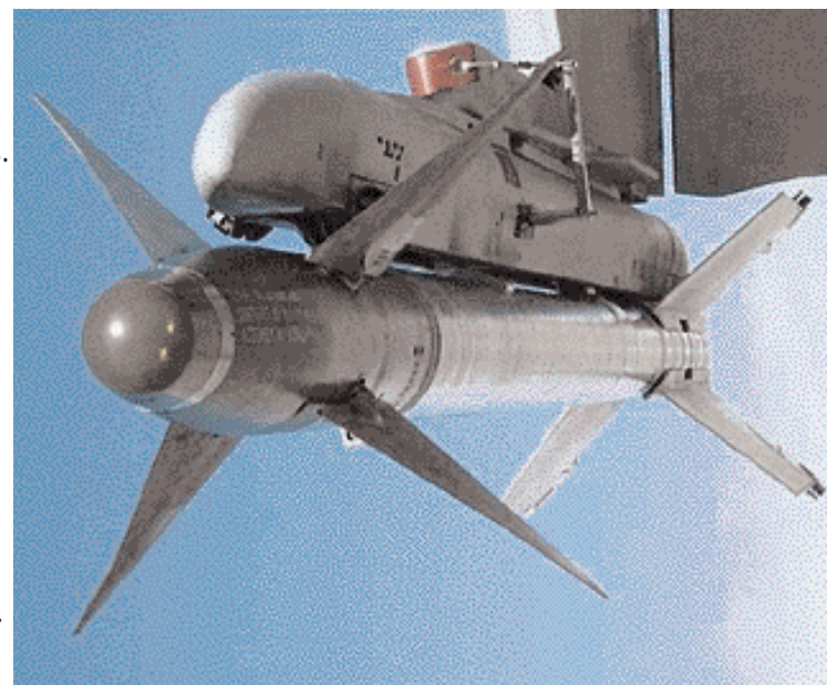
Flight Ready—the composite motor case mounted on an F/A-18 prior to a captive-carry flight.
